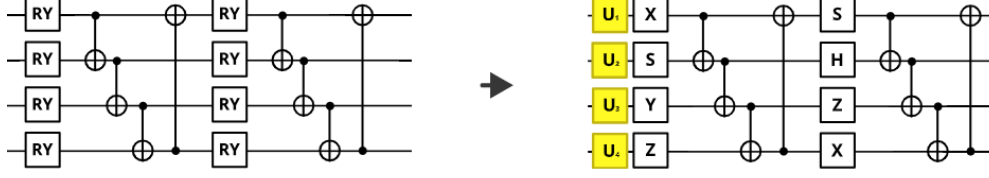
FIG. 2. Workflow of the proposed machine learning quantum error mitigation protocol. Training data are generated from efficiently simulable Clifford and near-Clifford circuits and used to train a regression model that predicts noiseless expectation values from noisy measurements.
